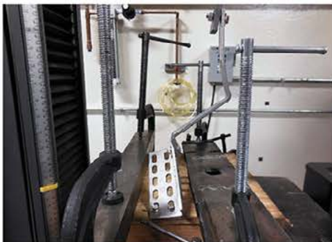
Photo 3: Typical Failure Mode - Fastener Pullout
