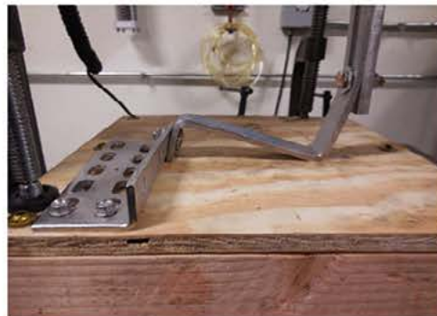
Photo 8: Typical Failure - Contact with Plywood
