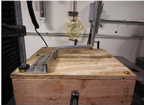
Photo 5: Compression Test Setup
