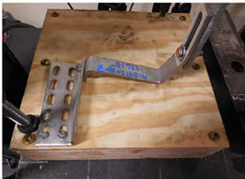
Photo 7: Hook Contact with Plywood
