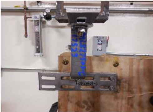
Photo 9: Shear Test Setup
