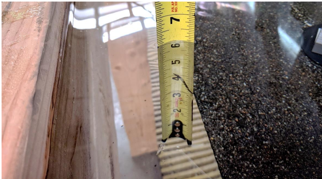
Photo No. 4 The water level was maintained at 6" for 7 days
